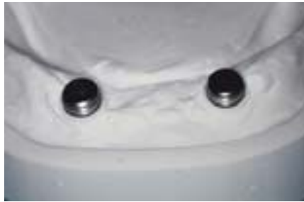
11. Metal-processing caps and spacer rings positioned on replicas.
